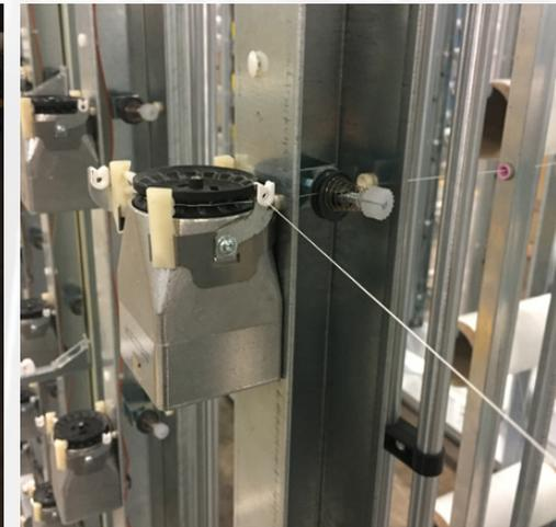
At the heart of the system is the touch screen, which allows operators to program every end with its individual tension, if the style requires. The system also monitors tight and loose ends where deviations to the pre-set tensions can be programmed based on your material's needs. Dynamic balloon control and crepe-type pretensioners are all available for your high-tech applications. The creel allows us to run 336 ends with a maximum spool diameter of 12" (305 mm).
